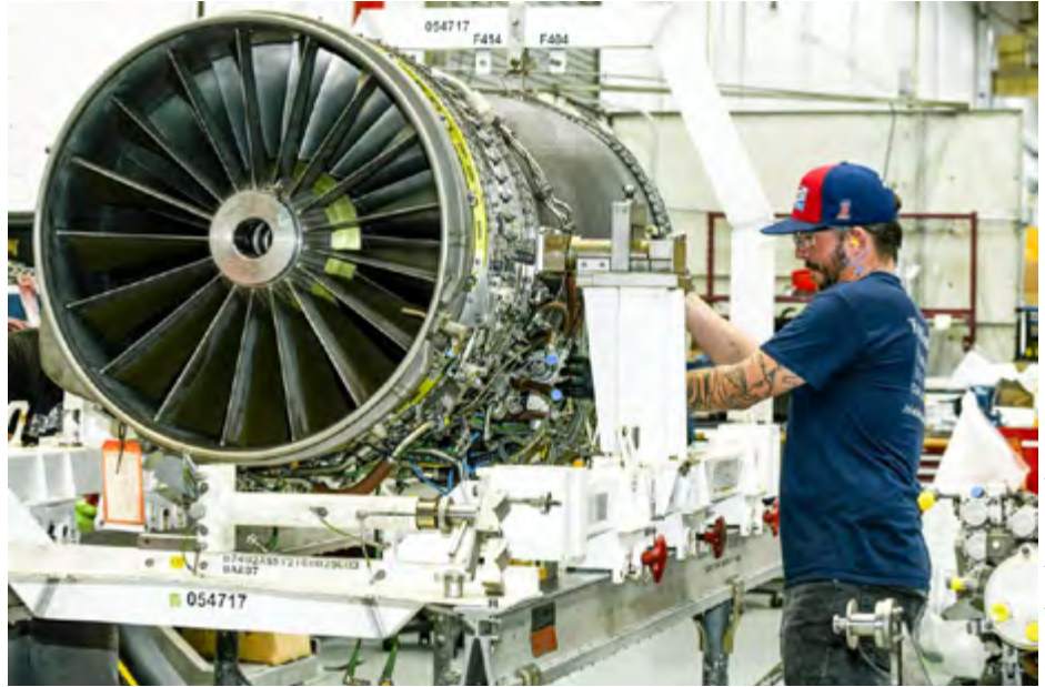
Aircraft Mechanic Michael Pucket installs a fan geometry actuator on an F414 engine.
