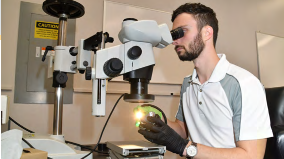
Latane Mason, a materials engineer at FRCE Materials Engineering Division, examines a fractured surface using a stereo microscope.
