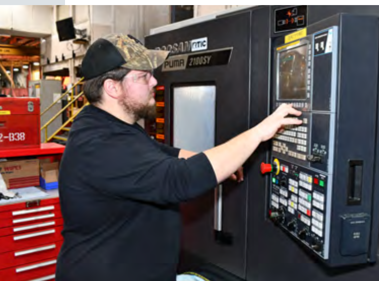
Dustan Brown, a machinist in the Manufacturing Machine Shop at Fleet Readiness Center East (FRCE), monitors progress of one of the depot's computerized numerical control lathes as it machines an offset pin for use in an AV-8B Harrier.
