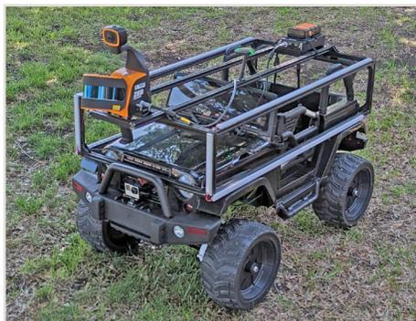
*U.S. Army Corps of Engineers Fort Worth District Geospatial Services Section constructed a remotely operated vehicle that can carry a hand-held LiDAR unit. The vehicle can carry the LiDAR unit into areas that may be unsafe for a human to enter.*
