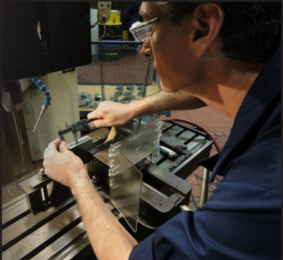
Toolmaker Ken Brink measures a work piece on a Computer Numerically Controlled (CNC) milling machine with digital vernier calipers. Engine lathes are used to produce cylindrical shapes of all types and are the metal cutting machines most commonly associated with machine work.
