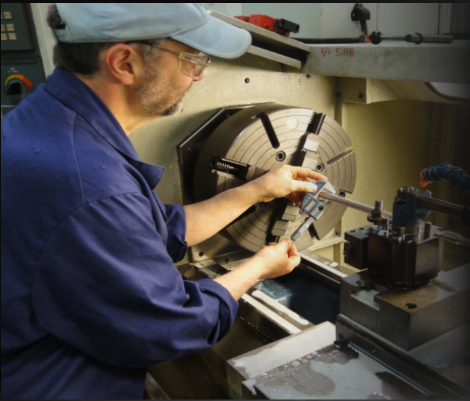
Toolmaker Jim Oswald uses a digital micrometer to measure an outside diameter on a Computer Numerically Controlled (CNC) engine lathe. (Shop 31 photos by Dennis Casteen, Code 931 Machinist.)
