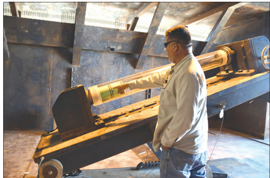
“The fabricators, welders, everybody that you see here, pitched in,” remarked Pablo Villalobos with the Targets Shop under Threat Systems. He estimates the table weighs 10,000 pounds and is used to elevate the ballistic simulator he’s pointing towards.
