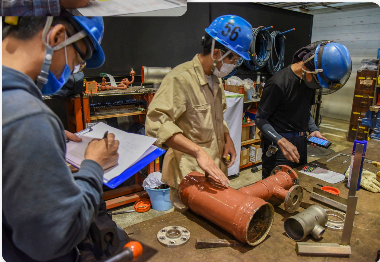
(Right) YOKOSUKA, Japan (Oct. 30, 2020) – Personnel from the pipefitting shop (X56) produce drawings and take measurements using a fraction calculator to fabricate sea-water pipes and pipe fittings.
