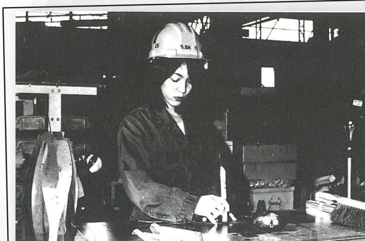
YOKOSUKA, Japan (circa 1997) – Ship sheetmetal worker Sanae Saito (X17) etches a line on an aluminum sheet for fabrication of a ventilation duct elbow for USS Blue Ridge (LCC 19). (Photo source: SRF Trade Development Program Class 9 Graduation Yearbook)
