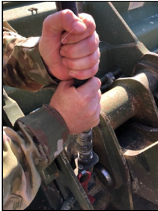
Ensure hose couplings click tightly to prevent leaks
