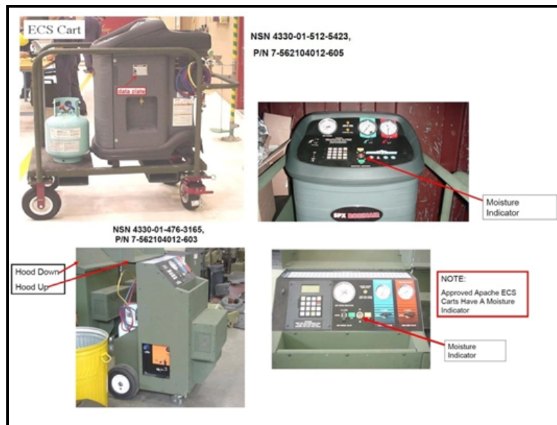
ECS carts that can be repaired (Right click and open in new tab to view larger image)
