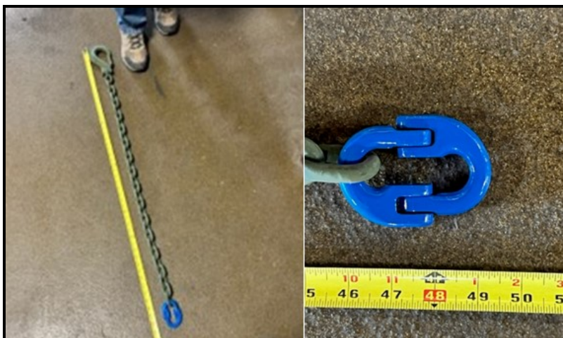
Measure to ensure safety hook to detachable link is 50 inches
