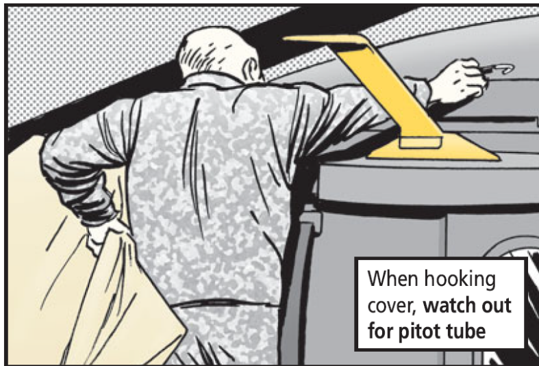
When hooking cover, watch out for pitot tube
