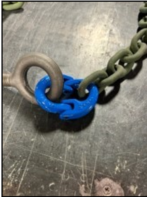
Detachable link connects safety chain to water trailer eye bolt
