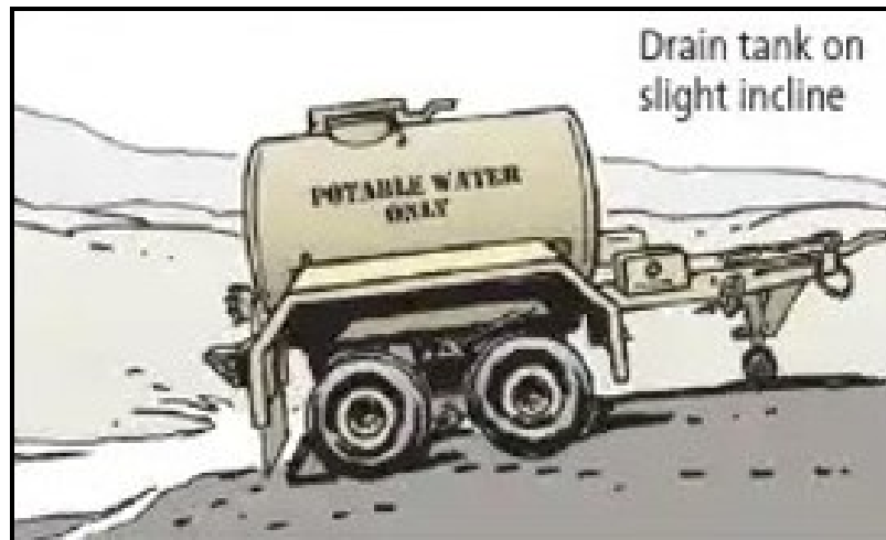
Trailer on incline enables water to drain through the drain plug completely.
