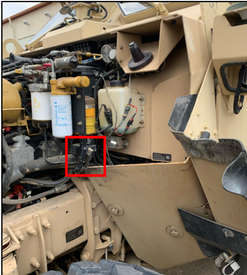
10-AMP fuse on C51 connector in engine compartment
