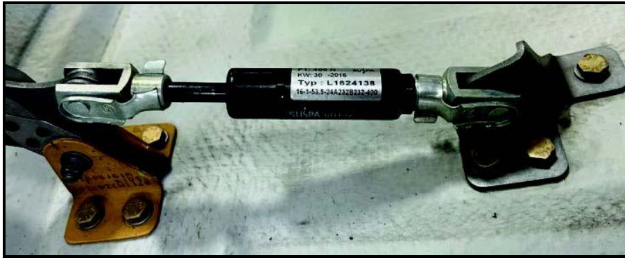
Excessive play means wrong hardware used
