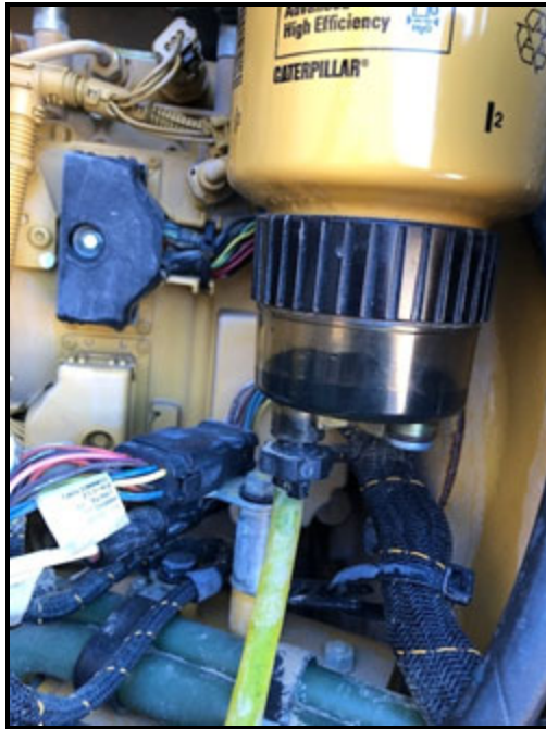
Turn drain-cock correctly to open
