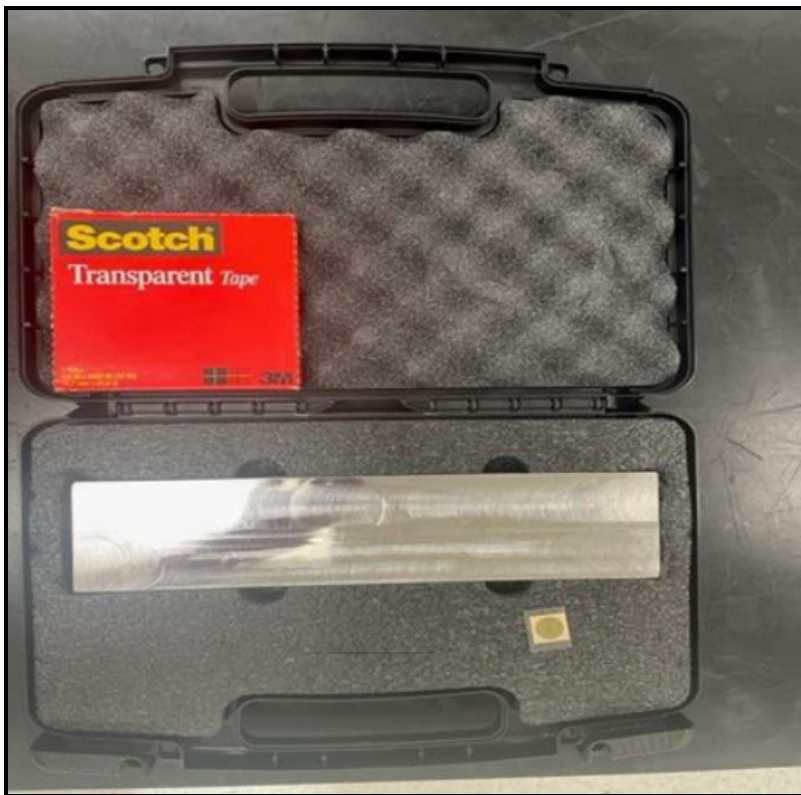
NDI shop set includes magnetic particle inspection kit
