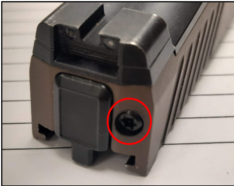
Correctly installed extractor tension pin; recessed in the slide
