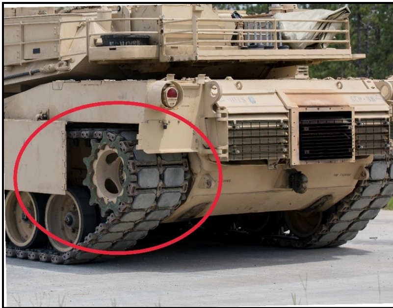
Missing rear mud guard (skirt #7) can lead to engine damage
