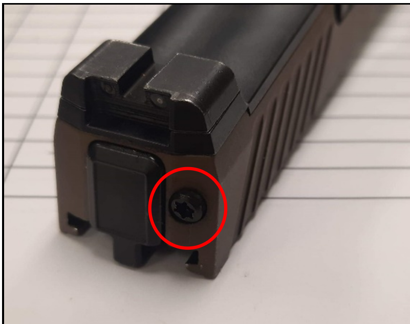
Incorrectly installed extractor tension pin; protrudes from the slide
