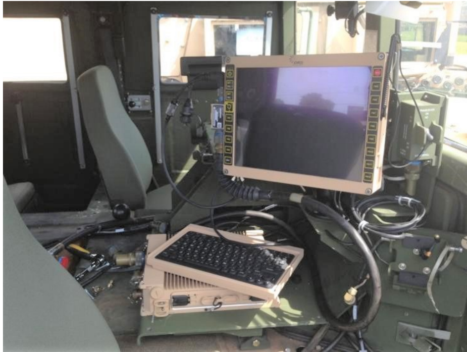
JBC-P MFoCS mounted in an M997A2 vehicle (Courtesy photo)
