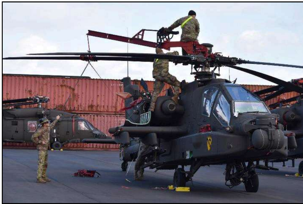
Return blade equipment to APMTT when aircraft movement complete
