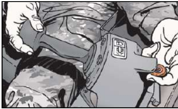
Lock parking brake to start engine
