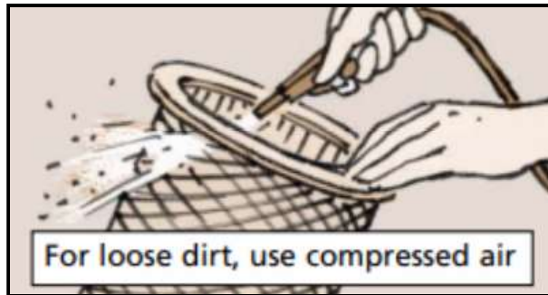
For loose dirt, use compressed air
