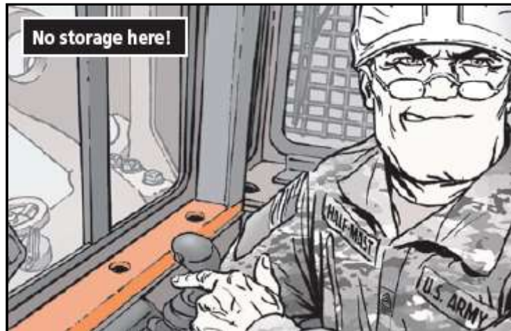
Don't use the area behind the winch handle for storage
