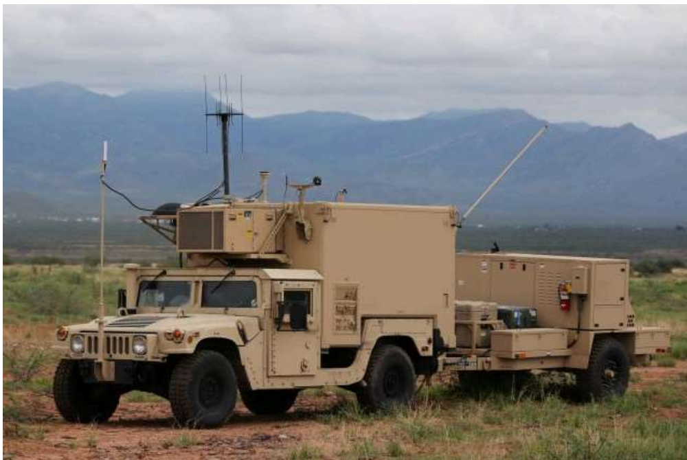
TGS mounted on HMMWV (Courtesy photo)
