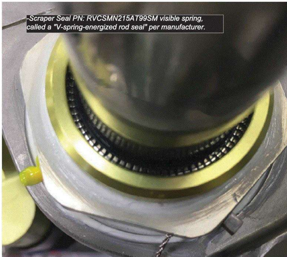
Another view of the scraper seal visible spring, also called a v-spring rod seal
