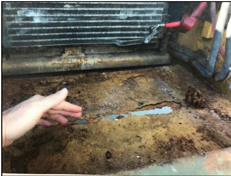
Corrosion in the HYEX battery box
