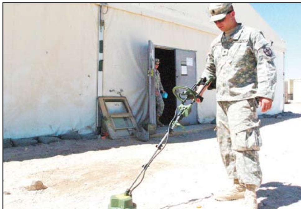
Spc. Jordan Manwill, a combat engineer with the 391st Engineer Company, uses the handheld mine detector to find objects in the ground at NTC.
