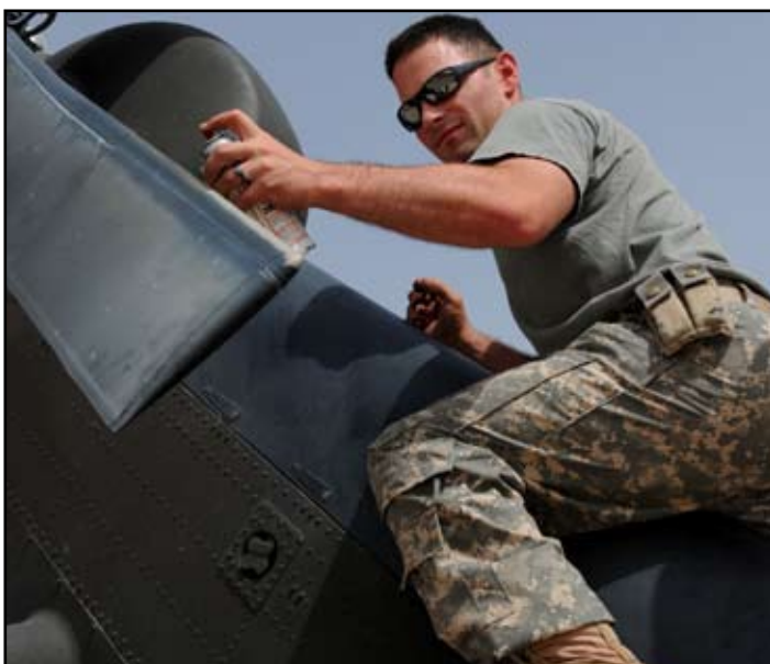
Photo by Spc. Cassandra Monroe, 135th Mobile Public Affairs Detachment Sergeant Ben Lind, a crew chief with Co. C., 3/1st Avn., 1st CAB, 1ID, sprays black paint on the tail rotor of a UH-60 Black Hawk helicopter to prevent erosion from sand, at COB Speicher, near Tikrit, Iraq, Aug. 9.
