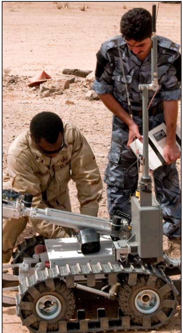
Explosive Ordnance Disposal 2 Rashid Graham, the senior bomb technician with EODMU Two, and Spc. Mustafa Gazwan, an EOD technician and robot driver with the IP, replace the battery of an Andros HD-1 robot during a training exercise, Aug. 7.
