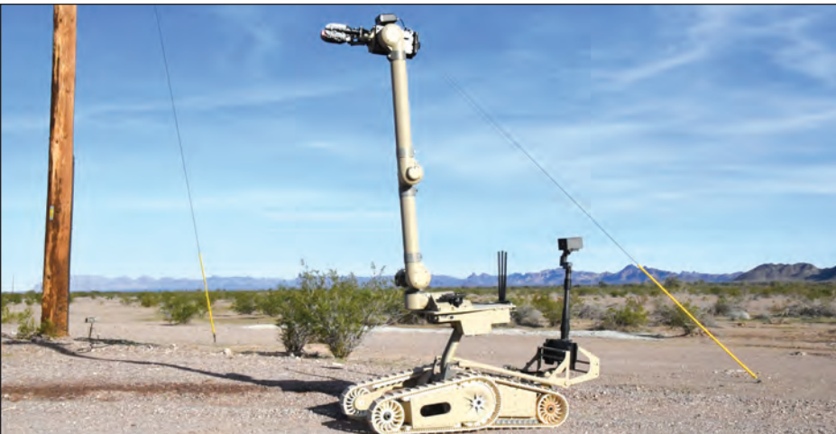
Technicians chose which robot to use depending on the situation and the weight of the item. The Kobra can lift a 155 round and reach higher. The Pacbot 525 has more maneuverability and it's lighter. The team utilizes the robots for various reasons which include, dragging the ammunition away to allow a safety buffer or lifting it for inspection. (Photos by Ana Henderson)
