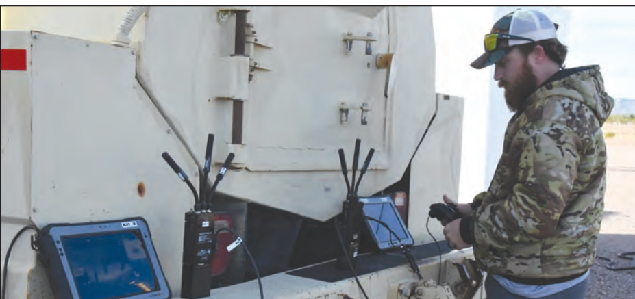
The tablets are used to see what the robot's 4k cameras are sending back and provide sharp color images. This is vital when looking for signs of arming which include color of lights and parts out of place. Ammunition Recovery Technician Brittan Forster is pictured operating the robots.
