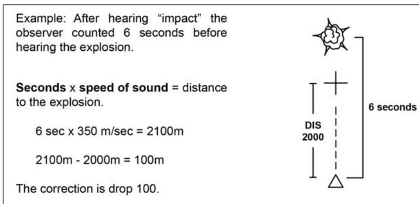
Figure 2 — Computing the Correction in Range
