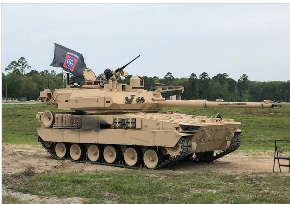
Enter the MPF. An approximately 42-ton tracked armored combat vehicle equipped with a 105mm gun, the M10 will be fielded to our light infantry forces and be able to press the attack, disrupting the enemy's intentions while still providing the speed and agility that have been the hallmark of light infantry since the days of the Marquis de Lafayette's service alongside George Washington in the American Revolution.
