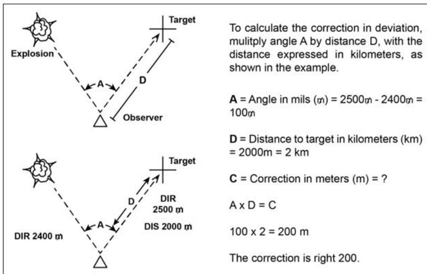
Figure 1 — Computing the Correction in Deviation
