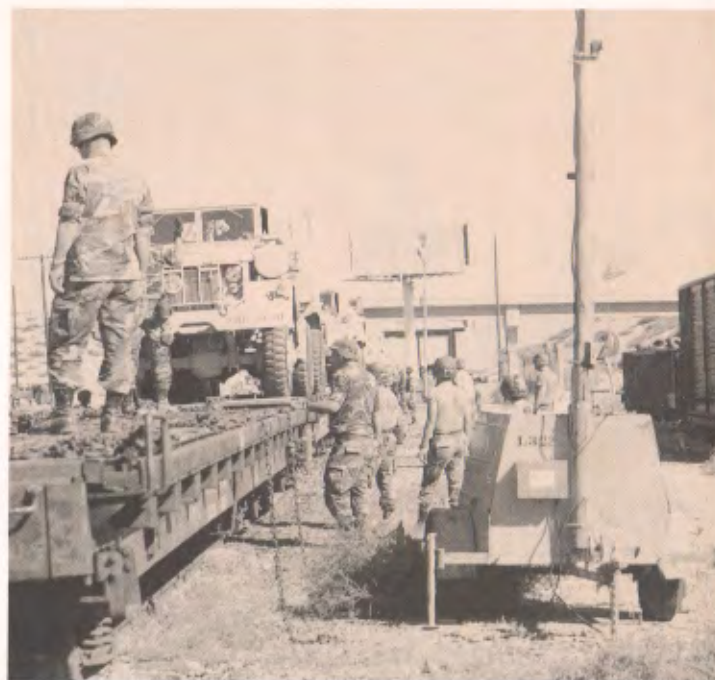
□ The use of portable, generator-equipped light sets (shown at right in photo above) permit loading operations to continue at night. Loading hazardous materials (below) requires special care. DCU expertise enables the loading to meet railroad standards (right).
