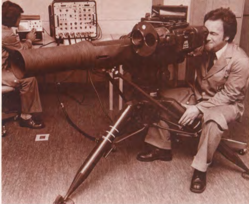
□ NAMSAs performs post-repair checks on TOW.
