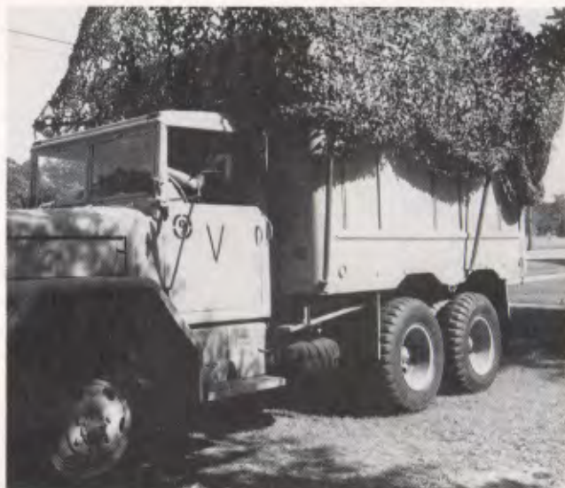
□ Camouflage netting resting in welded brackets makes this vehicle ready to be moved or concealed.
