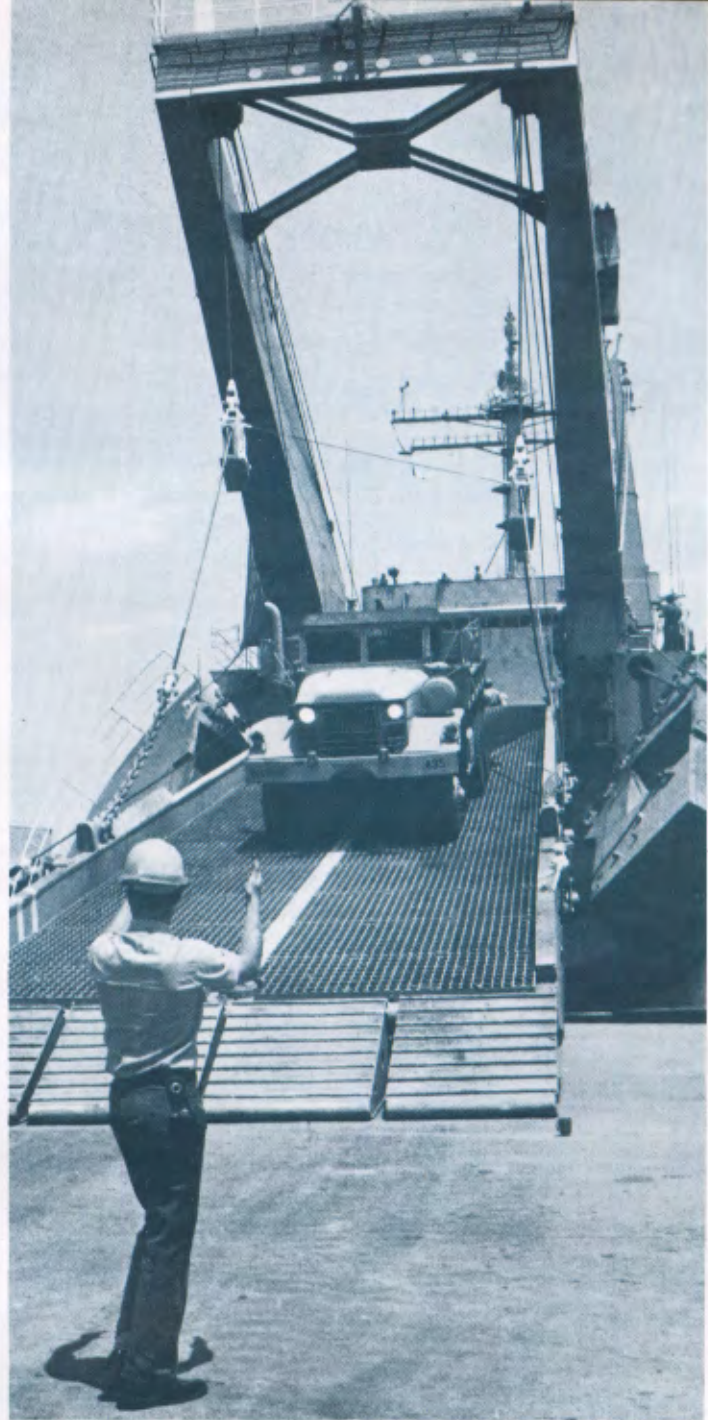
□ A Navy guide assists a driver in off-loading from the LST (above). After the LST's tank deck was emptied of its original cargo, it served as a passage to the dock for vehicles delivered by LCU's. An LCU (right), with its bow ramp locked onto the stern gate of the LST, transfers its load. After unloading, the LCU's were used to ferry vehicles in from the LPD, moored 12 miles away at the Savannah LASH (lighter, aboard ship) facility.
