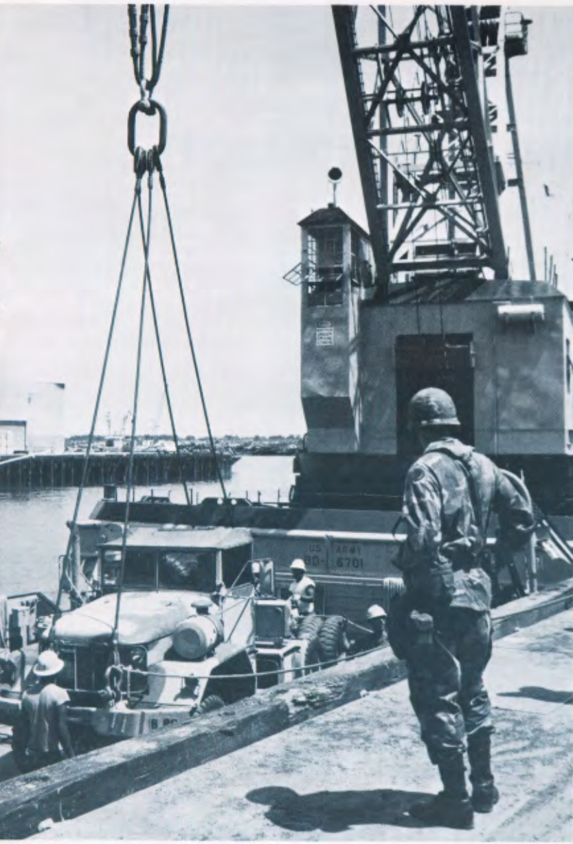
□ The Ranger —Army floating crane, BD-6701—lifts a 5-ton truck from the deck of an LCU. The crane from the 73d Transportation Company made the 3-day sea trip from Fort Eustis, Virginia, with the assistance of Army tug boats.
