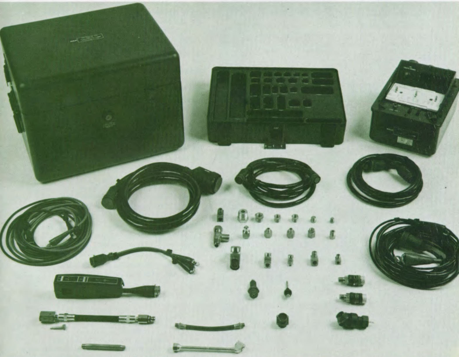
□ Components comprising the STE/ICE system.
