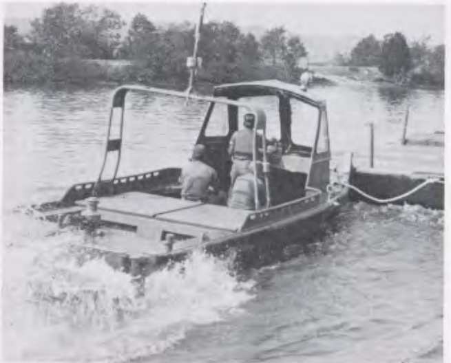
□ The jet-powered combat support boat pushes an interior bay of a ribbon bridge into position.
