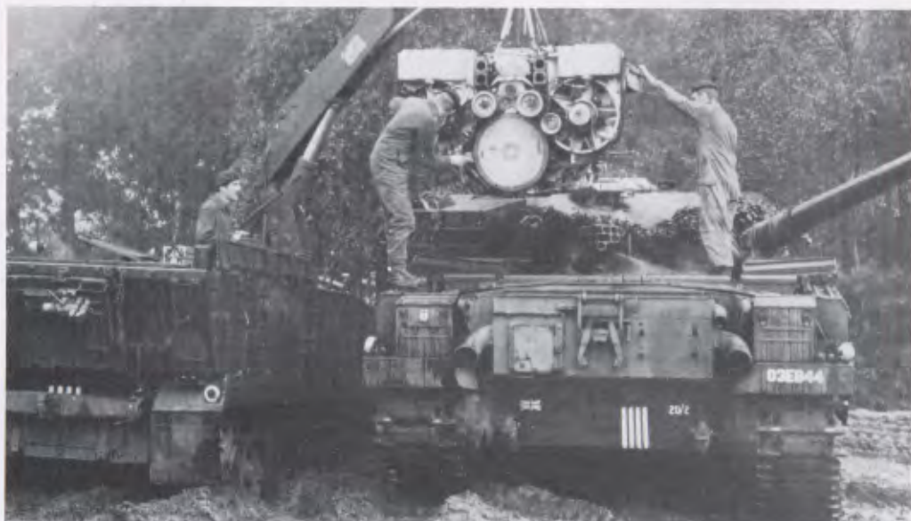
□ The British maintenance carrier crew uses a powerpack lift on this Chieftain main battle tank.
