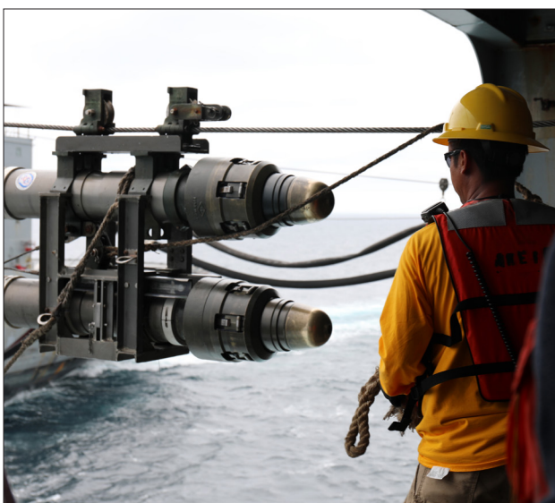
A view of the fuel nozzle from Military Sealift Command's fleet replenishment oiler USNS Kanawha (T-AO 196) as Civil Service Mariners serving on MSC's dry cargo, ammunition ship USNS Medgar Evers (T-AKE 13) bring it aboard during an underway replenishment-at-sea. (U.S. Navy photo by Bill Mesta)
