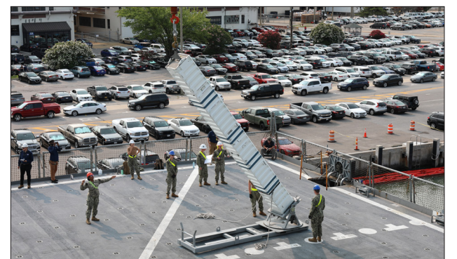
The crane from the dry cargo ammunition ship USNS William McLean (T-AKE 12) lifts simulated ordnance off of the flight deck for delivery to the Arleigh Burke-class destroyer USS Porter (DDG 78) during a Vertical Launch System re-arm demonstration held on Naval Station Norfolk, Aug 3. (U.S. Navy photo by Bill Mesta)
