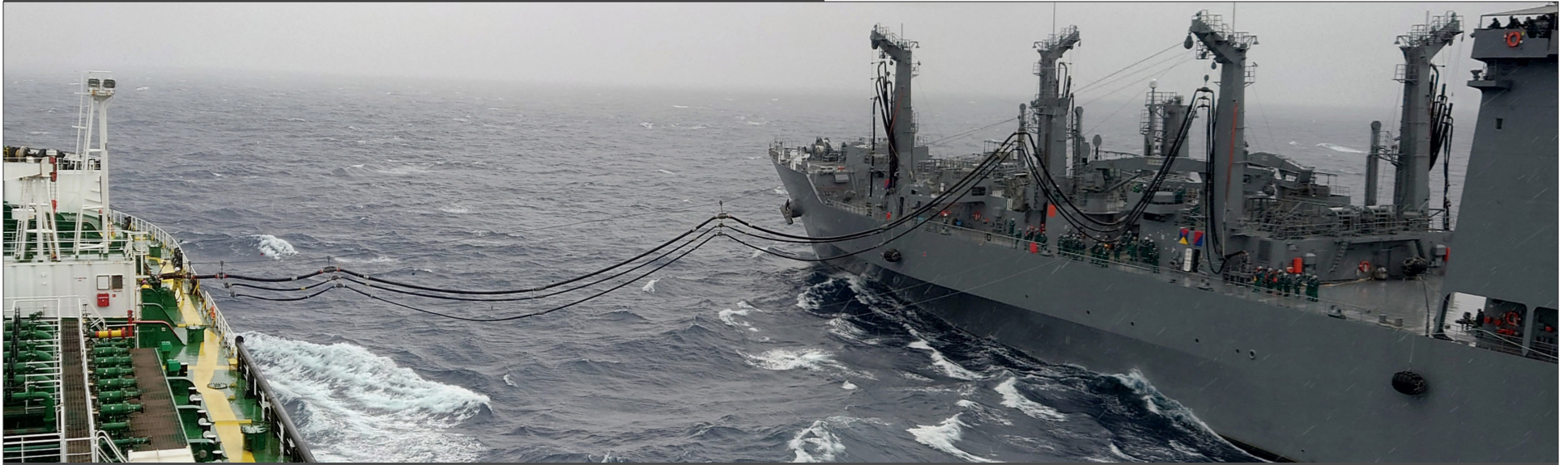
Military Sealift Command's commercial charter oiler MT Acadia Trader, left, connects fuel lines with Japanese Maritime Self-Defense Force oiler JM Oumi (AO-426), during ships qualification training, in which the ships performed a simulated consolidated cargo replenishment at sea, Oct. 8. (U.S. Navy photo)
