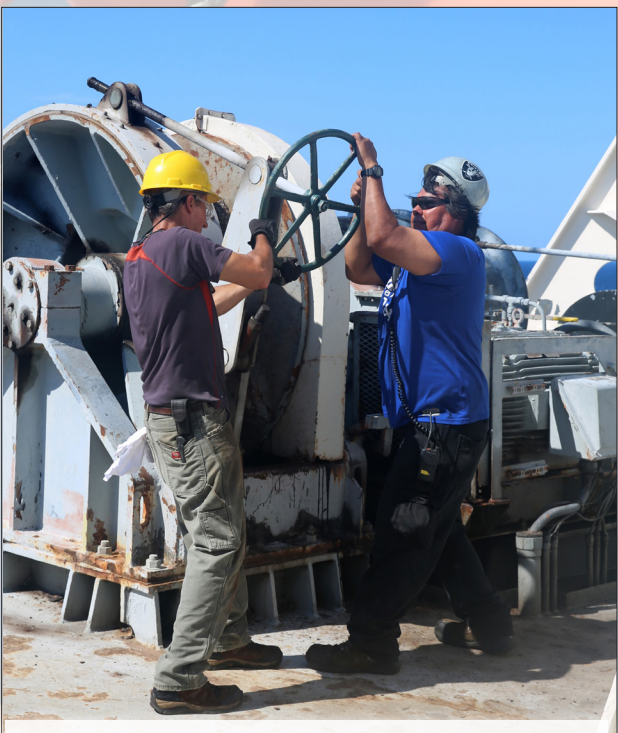
Able Bodied Seaman Lloyd LaBeach and Bosun Sam Yazı engage the anchor windless break aboard Military Sealift Command's container, roll-on/roll-off ship USNS SGT. Matej Kocak (T-AK 3005), Aug 18. Kocak was underway to perform sea trials. (U.S. Navy photograph by Bill Mesta)
