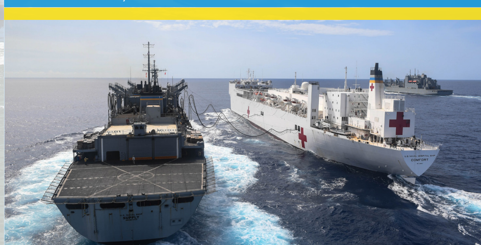
The Military Sealift Command hospital ship USNS Comfort (T-AH 20), center, conducts an underway replenishment with the dry cargo and ammunition ship USNS William McLean (T-AKE 12), left, and the fast combat support ship USNS Supply (T-AOE 6). (U.S. Navy Photo by Mass Communication Specialist 1st Class Ernest R. Scott)
