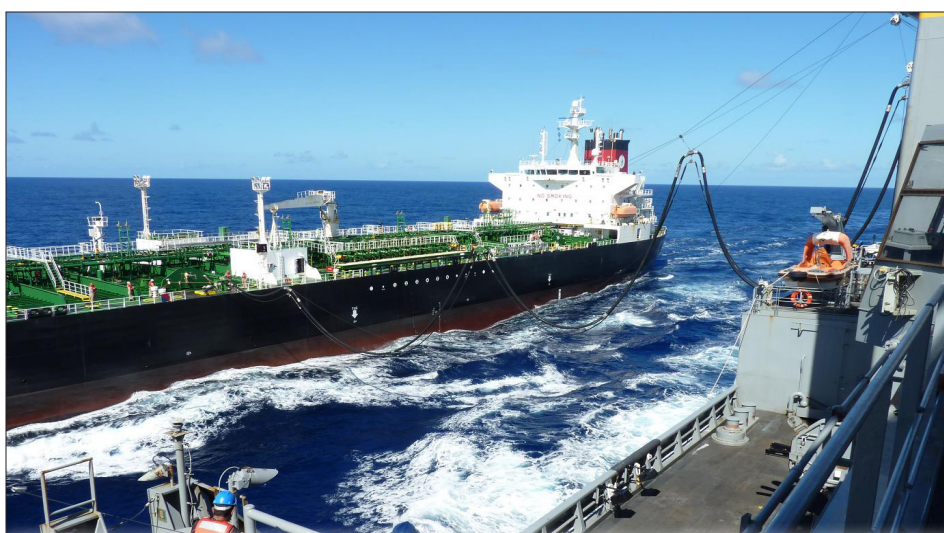
Military Sealift Command's dry cargo/ammunition ship USNS Matthew Perry (T-AKE 9) conducts a consolidated cargo replenishment CONSOL with the chartered motor tanker ship Empire State (T-AOT 5193), July 28. This was the first time a CONSOL has been conducted between a state class tanker ship and a dry cargo/ammunition ship. (U.S. Navy courtesy photograph)
