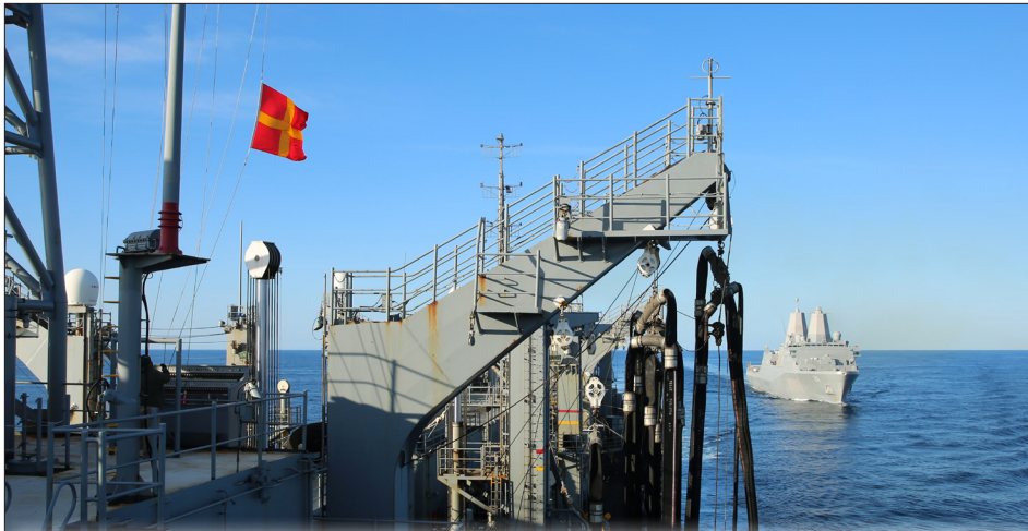
A civil service mariner attached to Military Sealift Command's fast combat support ship USNS Arctic (T-AOE 8) changes the ROMEO flag signaling to the San Antonio-class amphibious landing dock ship USS Arlington (LPD 24) that it is ready to begin an underway replenishment at sea, March 24. (U.S. Navy photograph by Bill Mesta)
