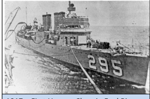
1917 – First Unrep - Close in Fuel Rig USS MAUMEE (AO2) - LT Chester Nimitz
