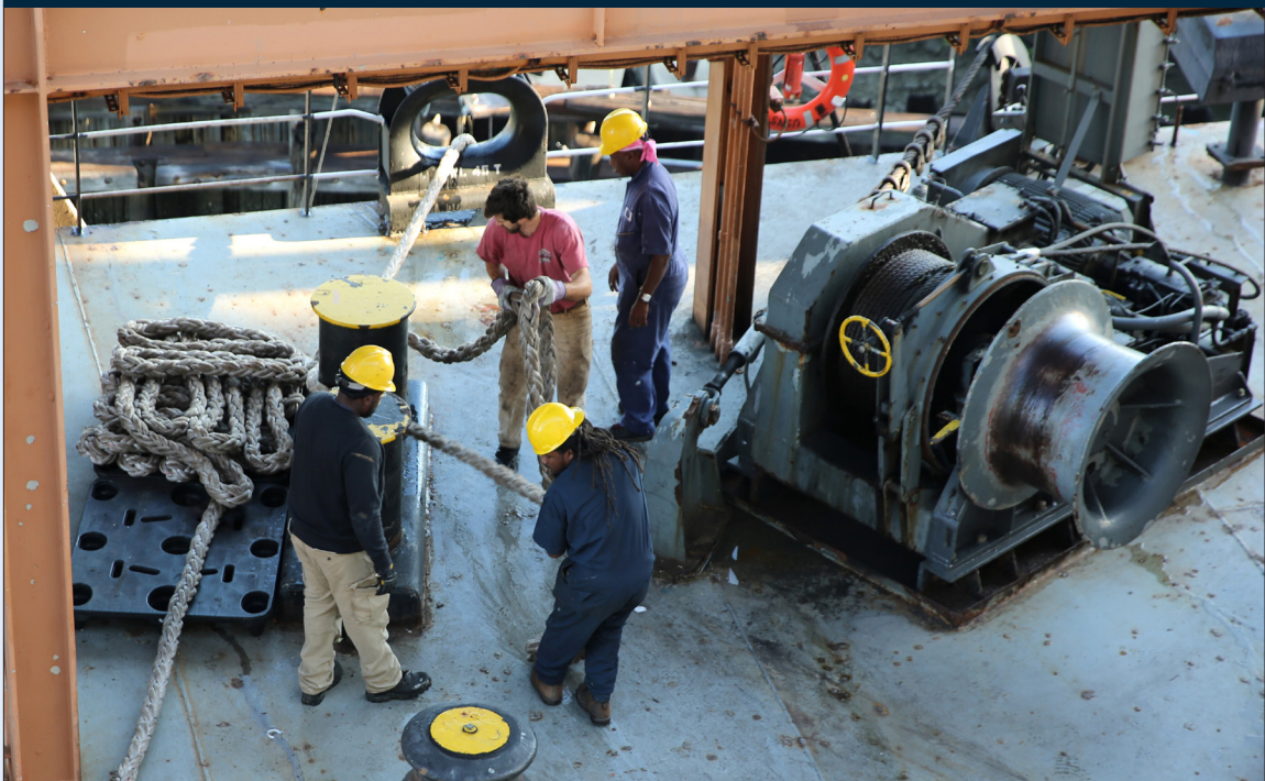
Contract mariners attached to Military Sealift Command’s roll-on/roll-off surge sealift ship USNS PFC Eugene A. Obregon (T-AK 3006) pull aboard mooring lines as the ship gets underway from Newport News, Virginia, Sept. 22. (U.S. Navy photo by Bill Mesta)
