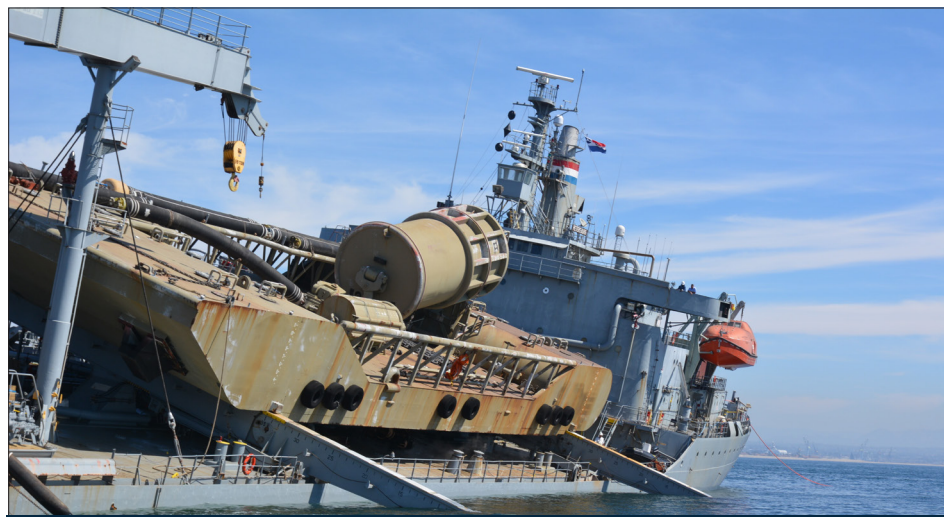
The Military Sealift Command tanker ship SS Petersburg (T-AOT 9101), sits in a 12-degree list as it successfully deploys a single-anchor leg mooring (SALM) buoy, the first of this type of exercise conducted in Southern California. The ship is participating in Arctic Expeditionary Capabilities Exercise 2019 off the coast of San Diego. (U.S. Navy photo by Sarah Burford)
