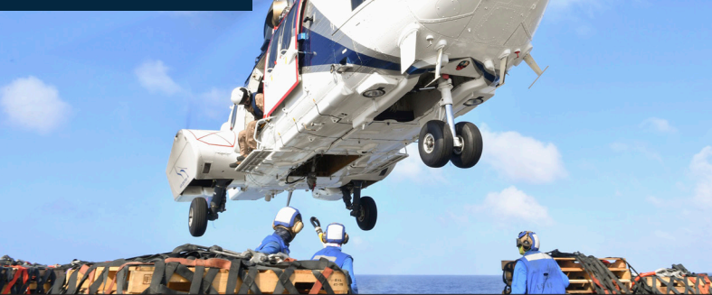
Sailors prepare to hook cargo to an Aerospatiale SA 330J Puma from the USNS Richard E. Byrd (T-AKE 4) during a vertical replenishment-at-sea. (U.S. Navy photo by Mass Communication Specialist 1st Class Toni Burton)
