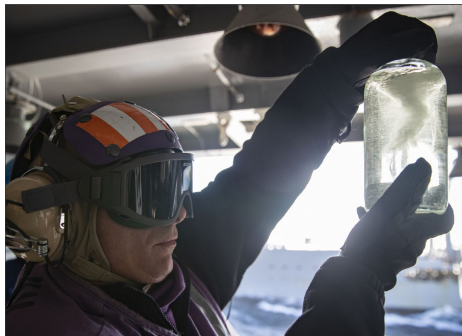
Chief Aviation Boatswain's Mate Michael Kyne, assigned to the aircraft carrier USS Gerald R. Ford (CVN 78) visually inspects a fuel sample during an underway replenishment at sea with the fleet replenishment oiler USNS Leroy Grumman (T-AO 195). (U.S. Navy photo by Mass Communication Specialist Third Class Joshua Murray)
