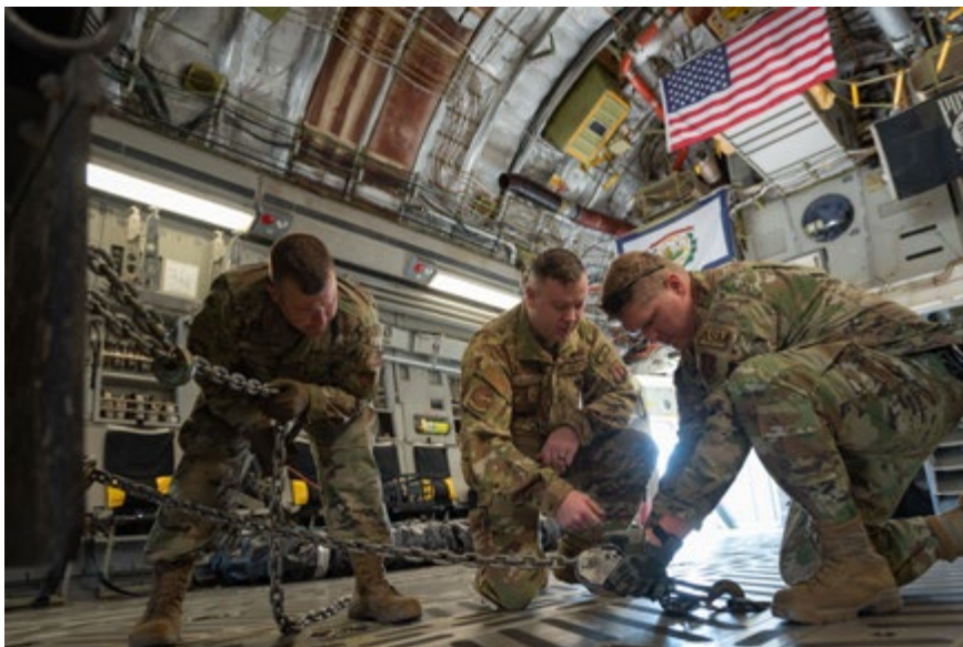
U.S. Air Force Staff Sgt. Raymie Roberts, center, 167th Operations Group loadmaster, instructs Tech. Sgt. Corey Chaney and Tech. Sgt. Daniel Barrow on how to tighten tie-down chains to secure a vehicle inside of a C-17 Globemaster III aircraft as part of a Multi-Capable Airmen (MCA) training at the 167th Airlift Wing, Martinsburg, West Virginia, Nov. 5, 2023. The MCA training focuses on developing competencies outside of the Airman's primary Air Force Specialty code, ensuring Airmen are ready for contingencies and are able to operate with varying levels of capacity and support. (U.S. Air National Guard photo by Airman 1st Class James DeCicco)
