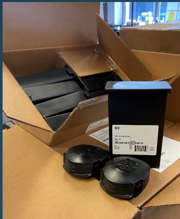
MOF-based filter prototypes for collective protection and general purpose mask. (NuMat Technologies, Inc., photo)
