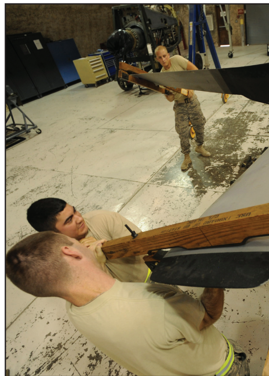
379 EMXS aerospace propulsion technicians work on a feather position here, June 8.
