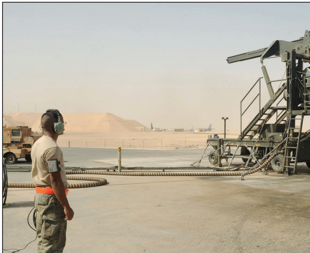
Senior Airman Francisco Rueda, 379th Expeditionary Maintenance Squadron, performs a fuel oil leak check on a C-130 engine test cell here, June 9.
