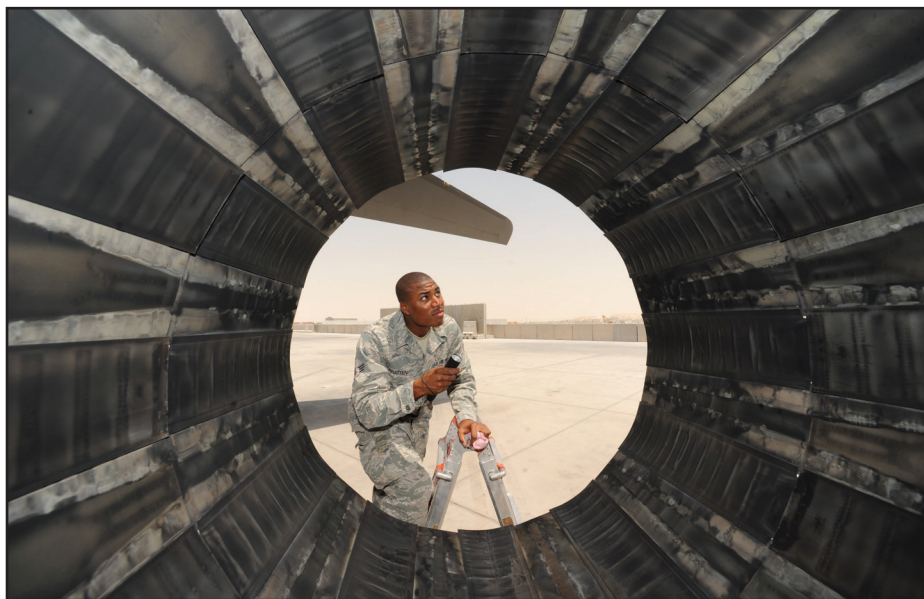
Senior Airman DeQuan McHatten, 34th Aircraft Maintenance Unit crew chief, performs a pre-flight inspection on a B1-B Lancer aircraft exhaust here, June 12.
