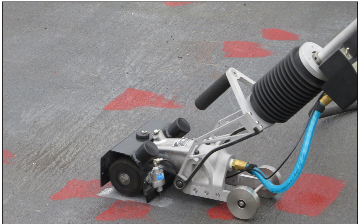
LEFT: Code 970 Mechanic Dionisio Dillard uses the Standup Abrading Machine (SAM) on the USS McKee (AS-41); ABOVE: The Standup Abrading Machine is an ergonomic device that is able to smooth out rough surfaces, including non-skid surfaces.
