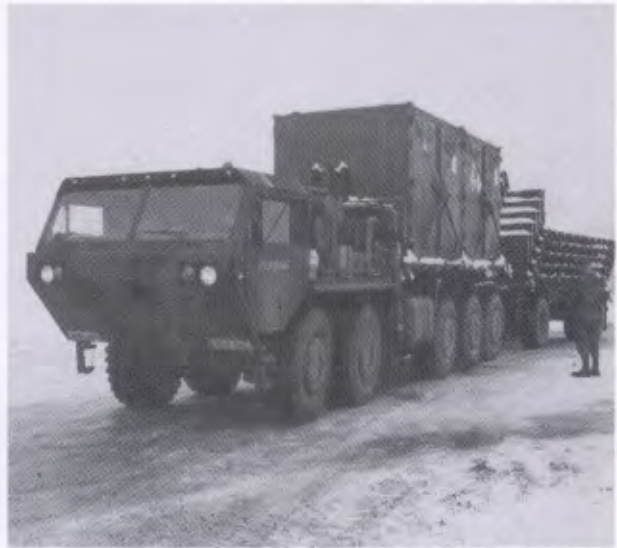
□ A driver uses the hydraulic load-handling system of the PLS to unload a flatrack (left). An M1075 PLS truck is ready to roll at the ISB (right).
