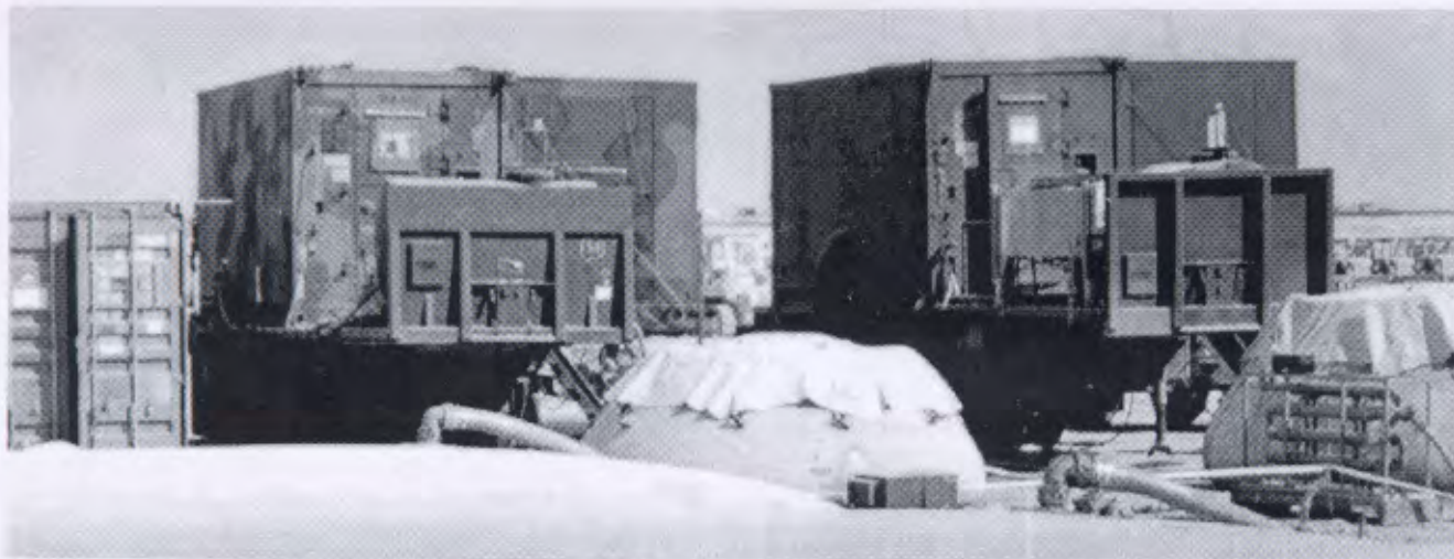
□ Both the water-packaging system (left) and the containerized ice plant (right) are housed inside expandable, trailer-mounted shelters and use water that has been processed through a reverse osmosis water purification unit.
