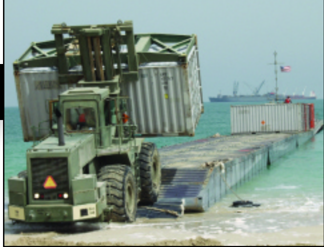
A rough terrain cargo handler unloads ammunition at Kuwait Navy Base during logistics-over-the-shore operations. Photo by Photographer's Mate Third Class Aaron Pineda, U.S. Navy, provided to Army Logistician by Captain Bobby Hart, 143d Transportation Command, U.S.
