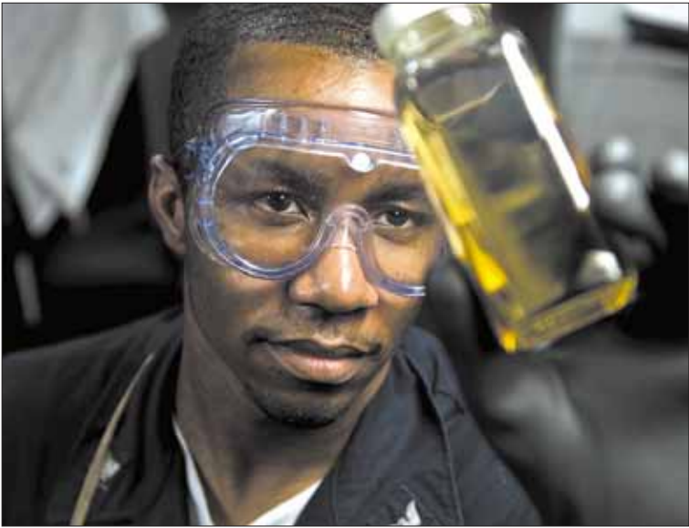
Machinist's Mate 3rd Class (SW) Dontra Brown from Seaford, Del., examines USS Nassau's (LHA 4) boiler fuel for sediment and water. Tests like these are run on every new batch of fuel, oil, and water the ship receives to ensure the boilers and engines run on the cleanest liquids possible.
