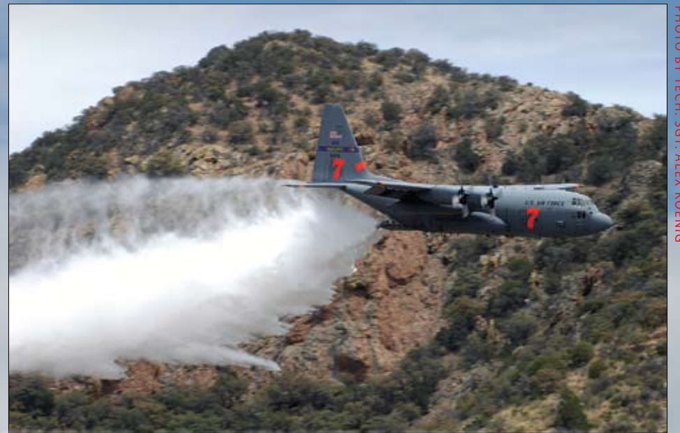
TOP: A C-130J Hercules from the 146th Airlift Wing based in Port Hueneme, Calif., drops water over treetops in South Carolina during the wing's annual Modular Airborne Fire Fighting System (MAFFS) training and certification April 26-30. INSET: A C-130J drops fire retardant near Tucson, Ariz., on May 8 to finalize its MAFFS certification by the U.S. Forestry Service.
