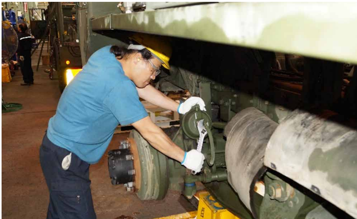
Min Su Yi, a mechanic in the Army Materiel Support Command–Korea's Tactical Wheeled Vehicle Team Four, tears apart a heavy expanded-mobility tactical truck fuel tanker. The vehicle's body, engine, transmission, and communications equipment will go to different work centers for simultaneous testing, repairs, cleaning, and paint.
