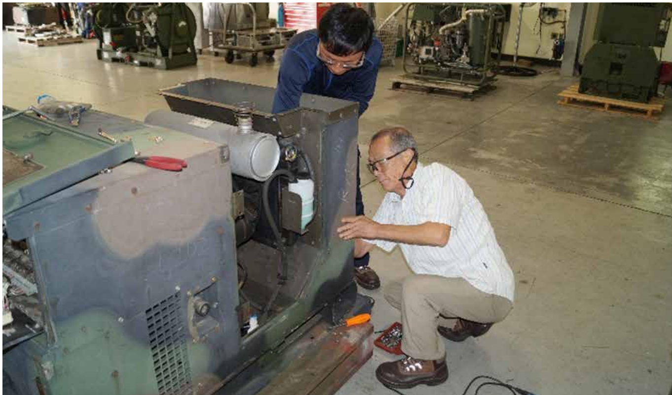
In the Major Assembly Division of the Army Materiel Support Command–Korea (MSC–K), Kil Song Kim performs a final quality inspection on a 500-kilowatt generator. Kim has been working for MSC–K since 1975.
