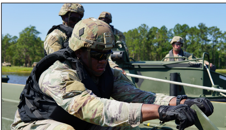
A Soldier constructs an IRB by joining the IRB bays and pumping the lever to secure the locks.
