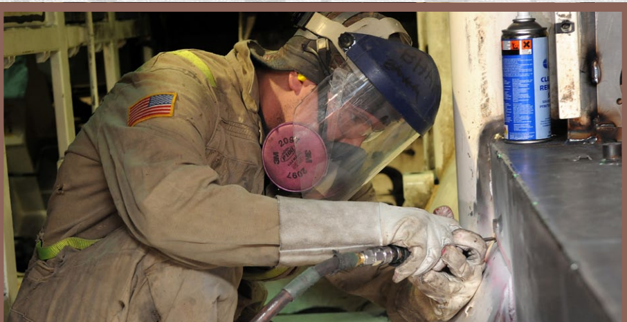
Tad Wendler, from Olympia, Wash., checks his welds for holes inside the Stryker battle damage repair facility at Camp As Sayliyah, Qatar, April 27. The Qatar base contains the only Stryker repair facility capable of complete structural overhauls in Southwest Asia. Wendler is completing his seventh battle-damaged Stryker. During the past 10 months, he has replaced punctured and warped plates, removed cracks and studied a 300-page configuration manual. (Official Army Photo/Dustin Senger)
