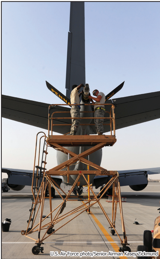
TOP LEFT: Tech. Sgt. Fredrick Mabry (left) and Airman 1st Class Daniel Winders (right), 379th Expeditionary Aircraft Maintenance Squadron crew chiefs, re-install a KC-135 boom nozzle here, Monday.
