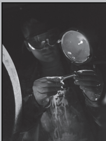
Staff Sgt. Richard Mabry, 379th Expeditionary Maintenance Squadron non-destructive inspection craftsman, conducts an inspection, in search of cracks, on a B-1B wheel bolt here, May 7.
