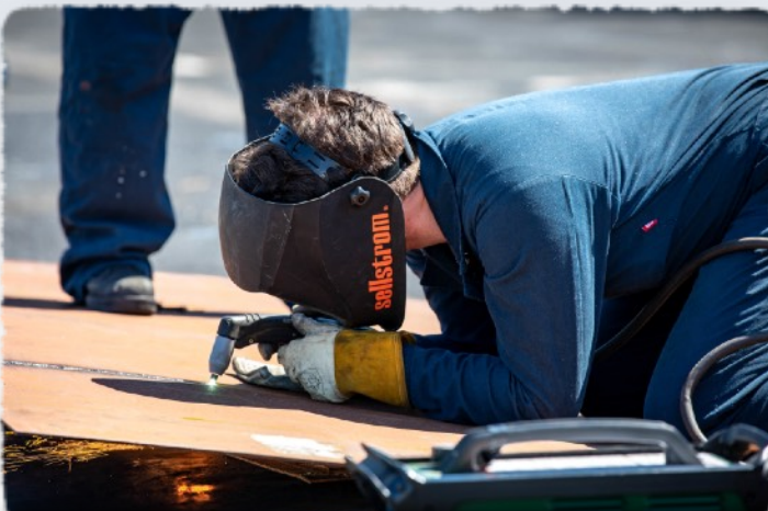
Hull Maintenance Technician 3rd Class Glenn Alexander, from Fort Worth, Texas, assigned to the San Antonio-class amphibious transport dock ship USS Arlington (LPD 24), cuts through carbon steel using a plasma torch during preservation work for mid-deployment voyage repairs in Rijeka, Croatia, July 6, 2022. (U.S. Navy photo by Mass Communication Specialist 1st Class John Bellino)
