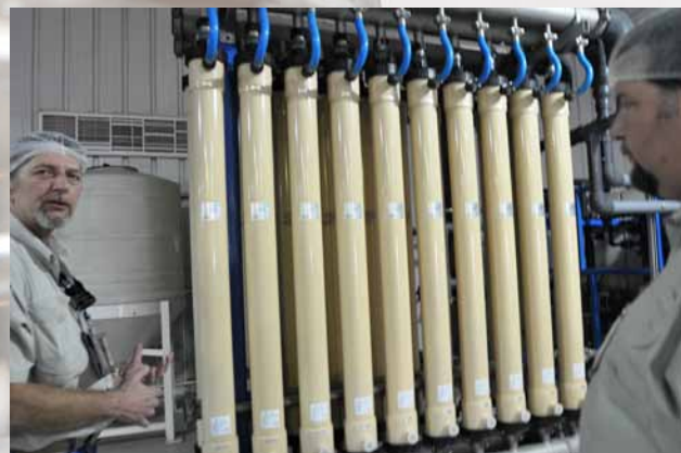
(right) Bruce McDougal (left) and Darren Woodruff (right) stand beside the Reverse Osmosis Filter membrane system inside the Oasis International Waters Bottling Plant on VBC.
