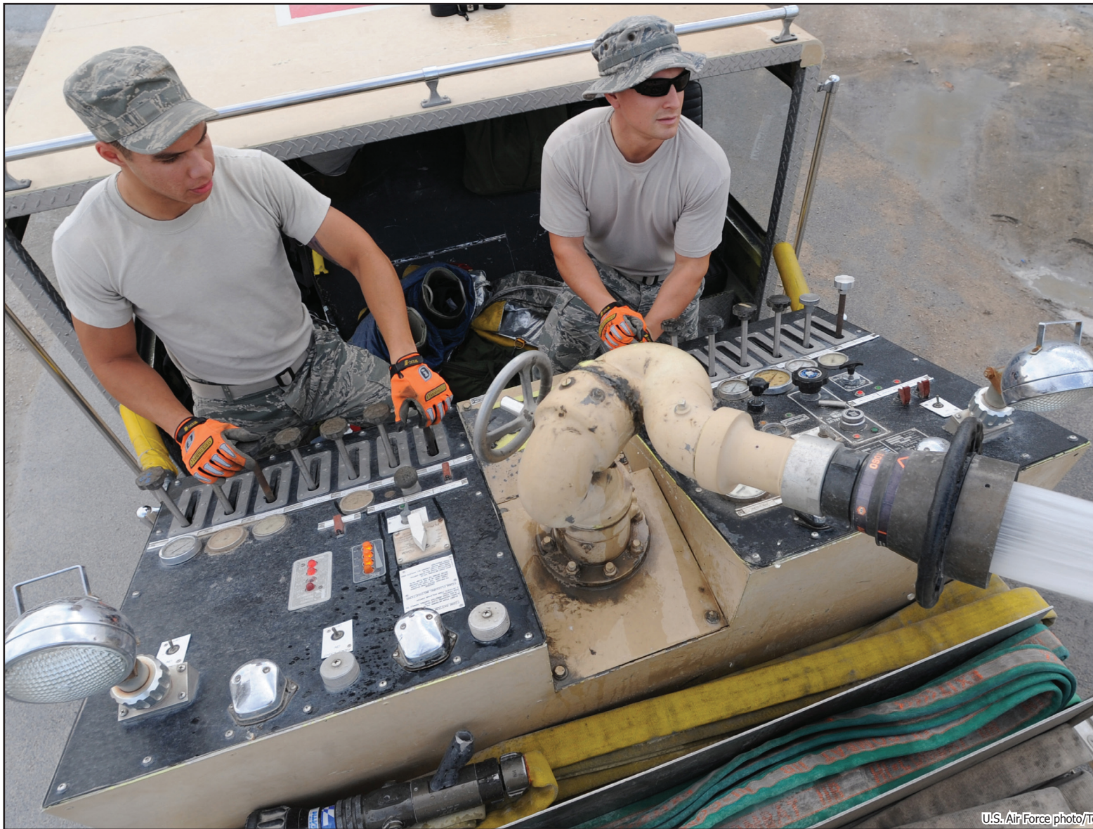
Airman 1st Class Ramon Betancourt (left) and Senior Airman Michael Waffle, 379th Expeditionary Civil Engineer Squadron, conduct an operational test on a firetruck deck gun here.
