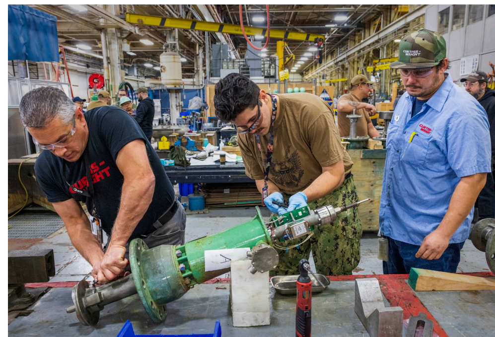
LEFT: Dylan Whaley, an electricians mate third class assigned to USS Theodore Roosevelt (CVN 71), assists with a valve repair in Shop 31, Machinists, Electroplaters & Toolmakers. Sailors were trained on repairs in a new collaboration between the shop and the ship. BELOW: Whaley, center, gets help disassembling a valve from Erik Kendrickson, right, a technician from contracting partner Curtiss Wright Fleet Solutions and John Devito, left, a technician from contracting partner Target Rock. (U.S. Navy photo by Wendy Hallmark)
