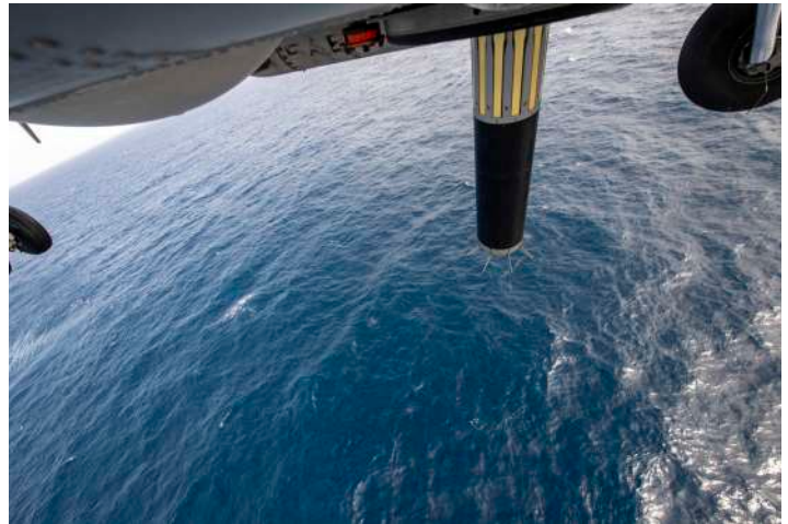
The sonar dipping transducer of an MH-60R Seahawk, attached to the "Saberhawks" of Helicopter Maritime Strike Squadron (HSM) 77, assigned to USS Shiloh (CG 67) is hoisted during an subsurface detection exercise evolution, June 23, 2021. (U.S. Navy Photo by Mass Communication Specialist 1st Class Rawad Madanat)
