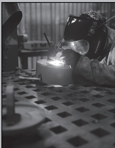
Staff Sgt. Rogelio Lopez, 379th Expeditionary Maintenance Squadron aircraft metals technology journeyman, welds an air filter housing for aircraft ground equipment here, Monday.
