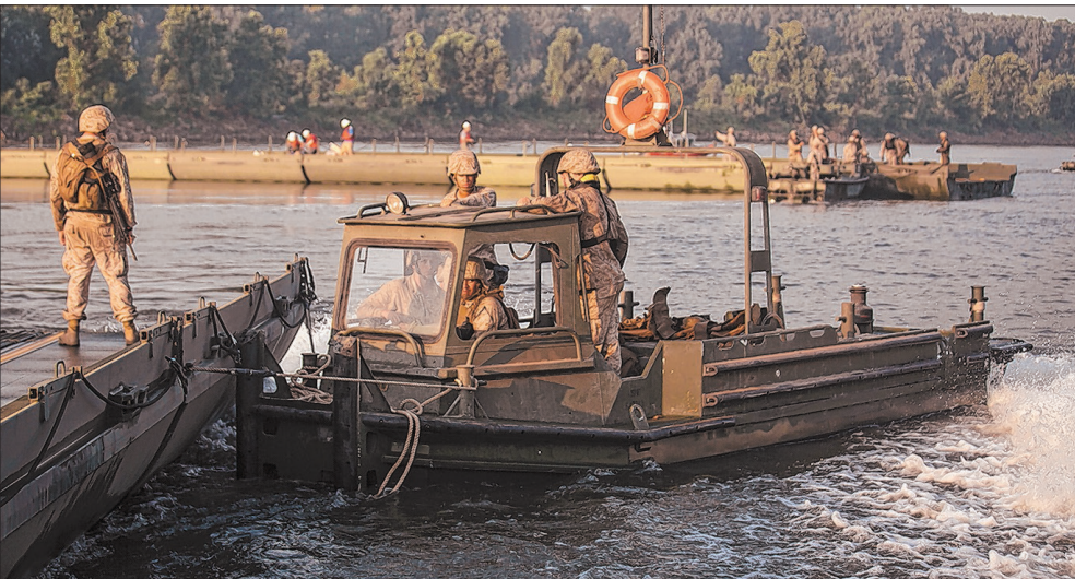
Photo by Cpl. Justin Updegraff Marines with Bridge Company, 8th Engineer Support Battalion and Bridge Co. B, 6th ESB maneuver an Improved Ribbon Bridge using a Mk3 bridge erection boat during Exercise River Assault on Fort Chaffee, Arkansas July 19.
