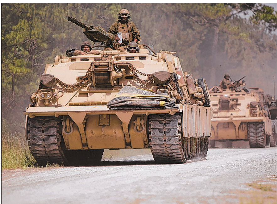
Marines with Company F, 4th Tank Battalion, drive to a landing zone to participate in an offensive and defensive exercise at Marine Corps Base Camp Lejeune July 19. The M88A2 Hercules has the ability to tow tanks that weight up to 70 tons, making it the first choice to recover tanks from the battlefield.
